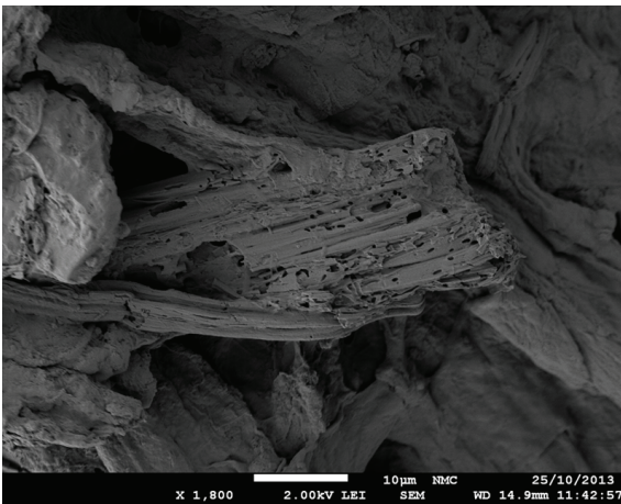
Fig. 7. SEM picture of the cotton fibre from the Vrouw Maria fragment. Photo: A. Nykänen.
