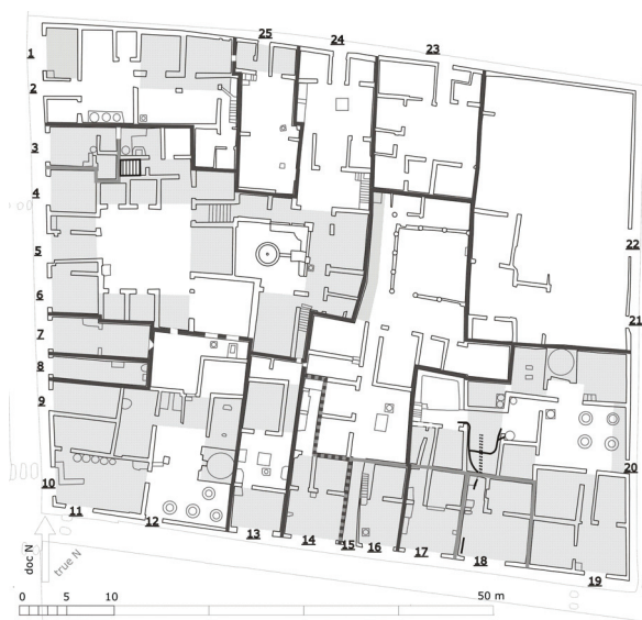
Figure 7. Shared structures between units in city block IX.3. Windows piercing walls between units are in white, a shared cess pool between Units IX.3 and 5 is striped, a shared water pipe between Units IX.3.18 and 19–20 is shown as a black line and a drain shared by them is marked with broken black lines. The extension of upper floors in each unit is indicated in light grey and the borders of units on upper floor levels are indicated in mid-grey (compare Fig. 6 showing the borders of units on the ground floor level). Unit clusters indicating common ownership are bordered in dark grey. The common ownership of Units IX.3.14 and 15 is not clear, which is indicated with a broken line. EPUH/Maija Holappa & Heini Ynnilä.
