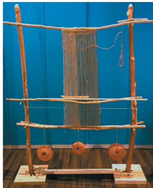
Figure 4. The loom measures 165 x 120 cm, with the base measuring 30 x 30 cm. Two loom weights hang from the sides of the warp, with the third one on the back beam to increase stability. The tubular tabby was started at the top. The lower beam sits on the supports in a “rest position” while work is paused. The bases are connected by a crossbar to fix distance between the poles and to give stability. (Photograph: L. Ariis)
