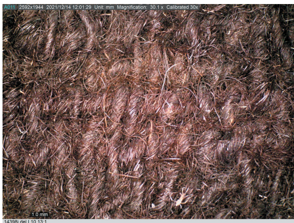
Figure 15. The woollen fabric in the doublet (Fragment 14398i), Dino-lite USB-microscope x30 magnification. (Image: J. Lindegren, SMTM)
