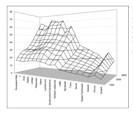
Fig. 2. Schematic overview of the temporal and spatial variation of the land-uplift on the Finnish coast. The graph shows the current elevation above sea level of locations that were coastal 1500 to 5500 calendar years ago.
